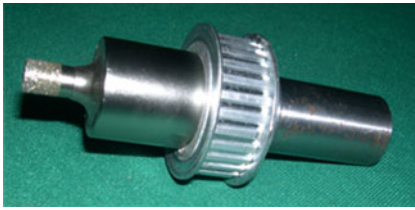
Fig. 1 Photograph of compound core-special drill
