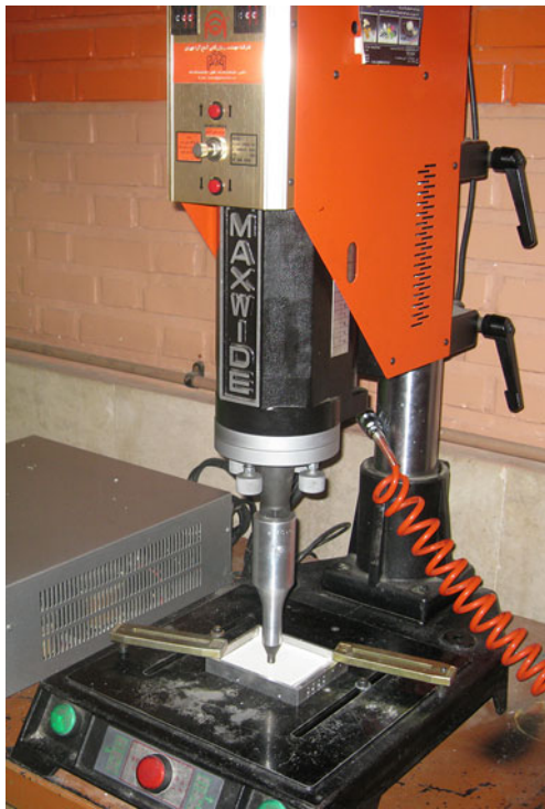
Fig. 4 15 KHz ultrasonic welding machine (Maxwide Inc.)
