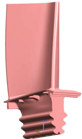
Fig. 10 CAD model of the turbine blade
