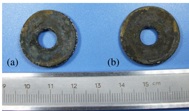
Fig. 11 TA15 titanium alloy rings deformed to about 42% height reduction with lubricant 1: a T=950^\circ\text{C} and b T=970^\circ\text{C}
