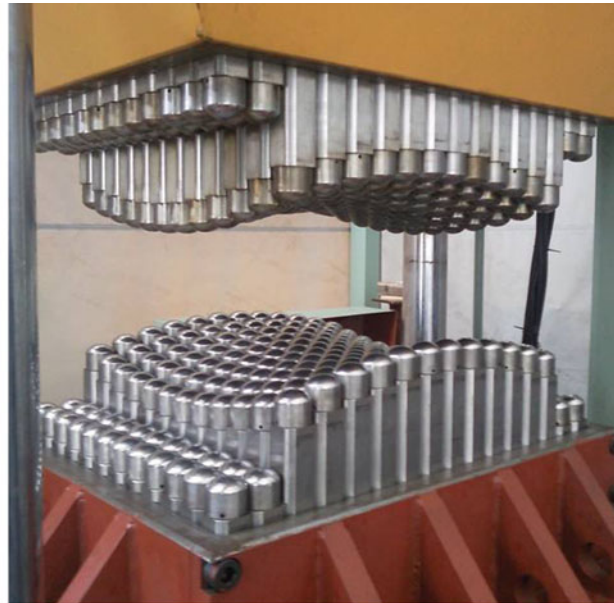
(a) Flexible die adjusted for saddle-type plate forming
