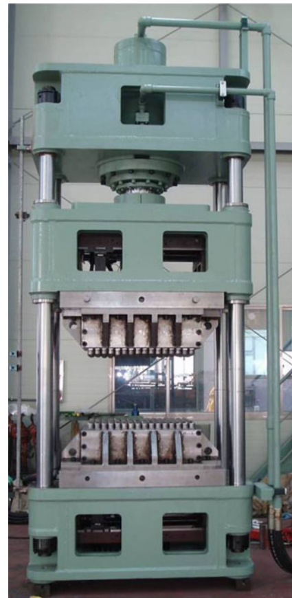
Fig. 17 Flexible forming apparatus with 2,000-kN hydraulic press
