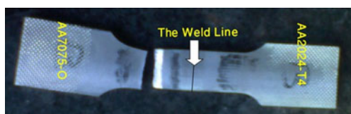
Fig. 14 A specimen which fractured at the BM of AA7075-O
