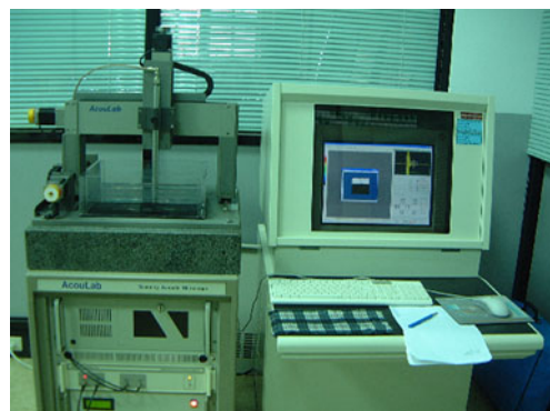
Fig. 6 Photograph of ultrasonic C-scan to measure the delamination
