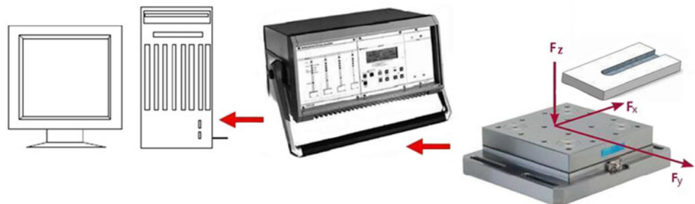
Fig. 5 Schema of measuring of the 3 orthogonal components of cutting force in the workpiece ( F_x , F_y , and F_z )
