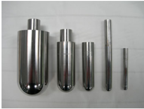
Fig. 4 The five different single-point forming tools that were utilised in the experiments. The tools have hemispherical tips and their radius varies from 25 mm ( leftmost ) to 4 mm ( rightmost )
