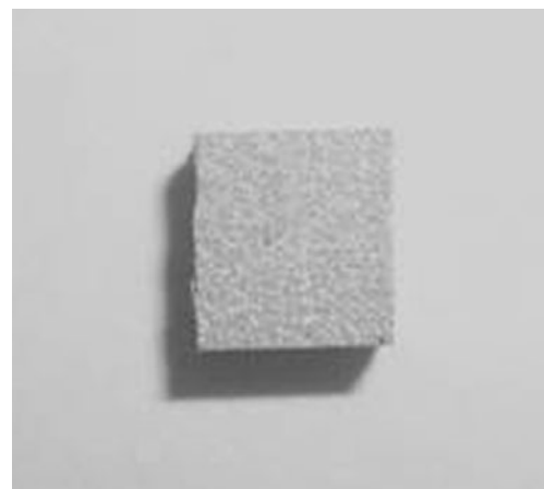
Fig. 6 Photograph of typical machined part of Al6063 with 5% SiC
