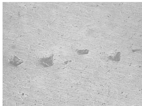
Fig. 3 Typical microscope image ( \times 400 magnification) of the composite material Al6063 with 10% SiC
