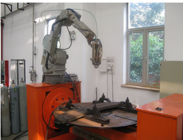
Fig. 2 The orbital welding of quenched and tempered low carbon low alloy steels
