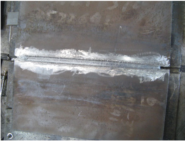
Fig. 1 The flat position welding of the quenched and tempered low carbon low alloy steels
