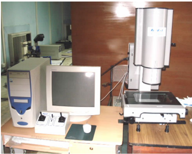
Fig. 3 Rapid 1 computer vision system for acquiring the images
