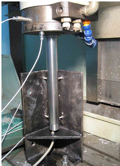
Fig. 7 The CNC center and sensors distribution
