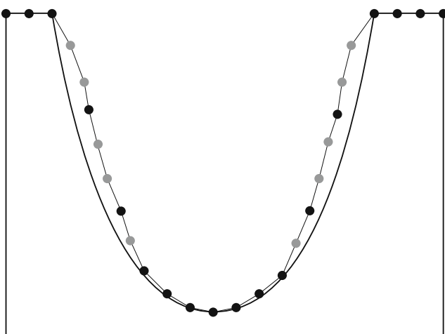
Fig. 5 Side view of c-space representation. The c-space is represented by discrete points lying on a regular grid connected to a mesh. If the z value of two adjacent points is too large, we insert further points in between. The points on the regular grid are colored black and the inserted points are colored gray
