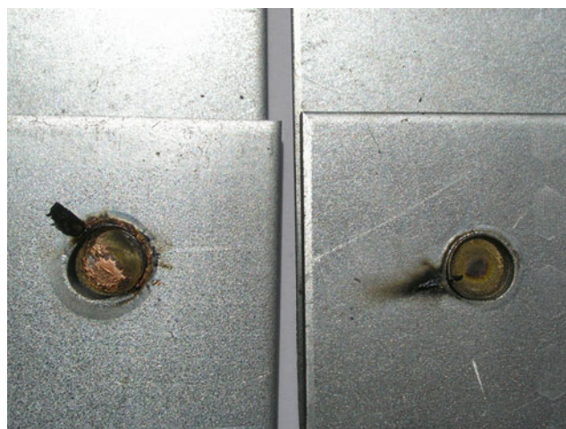
Fig. 13 A specimen welded without the application of the fuzzy controller (left) and a specimen welded with application of the fuzzy controller (right)
