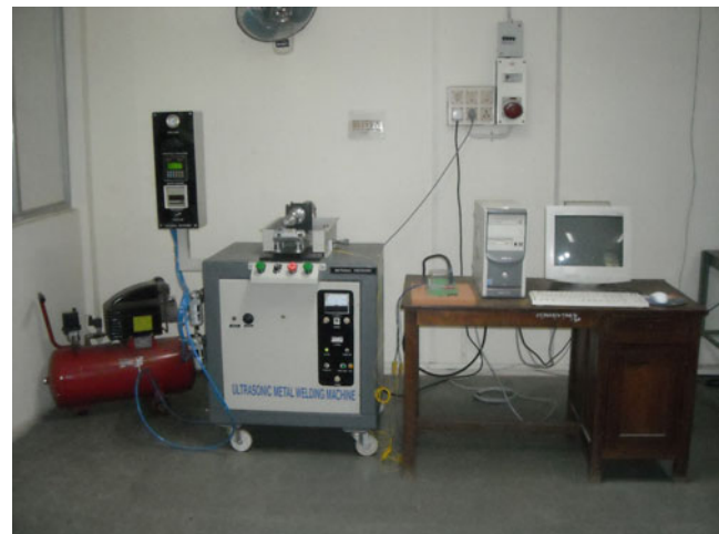
Fig. 2 Ultrasonic metal welding setup
