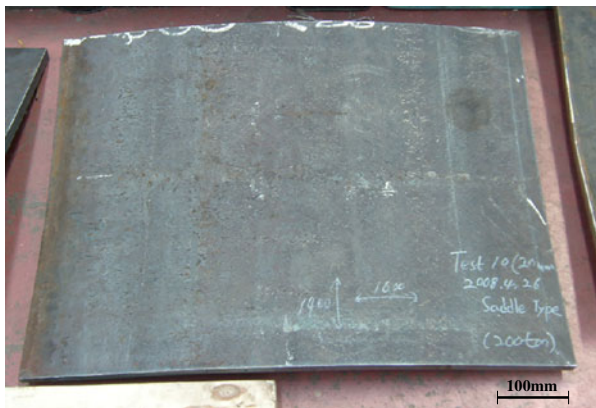
Fig. 23 A saddle-type curved plate formed by the flexible forming machine (800 mm × 600 mm × 20 mm)
