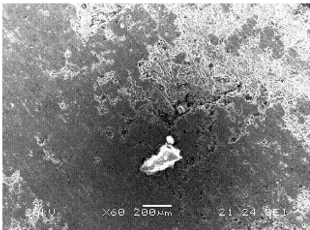
Fig. 7 SEM image of the surface of drilled hole (speed 160 rpm/feed 0.2 mm/rev, ×60)
