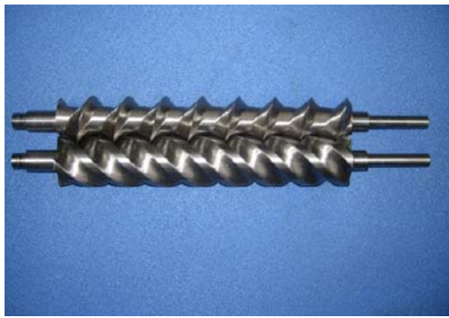
Fig. 9 Screw rotors machined by CBN grinding wheel
