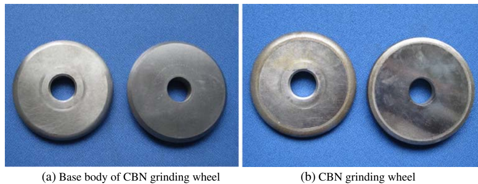
Fig. 7 CBN grinding wheel for machining the screw rotors
