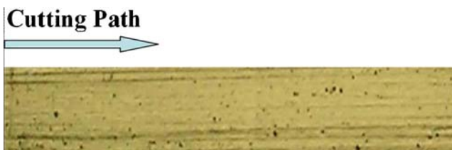
Fig. 16 Micrograph of finished surface by COP #2
