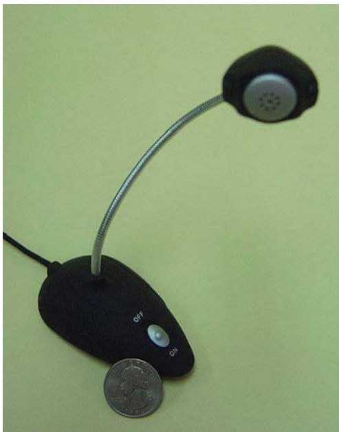
Fig. 8 Mini-microphone to acquire acoustic chatter signal
