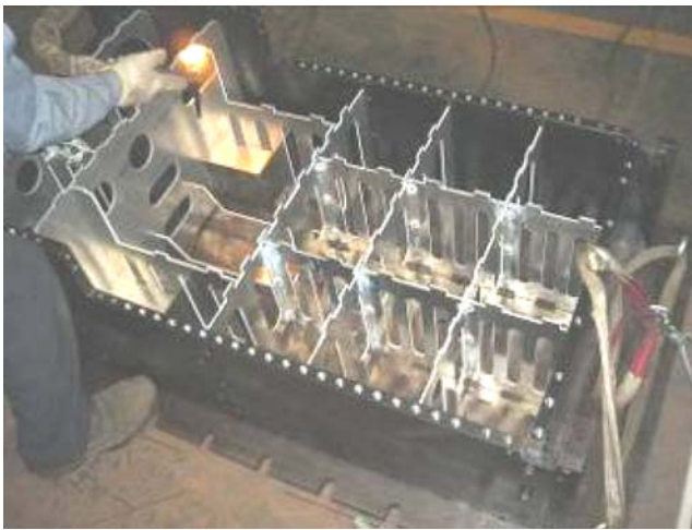
Fig. 17 Used for internal enforce assembly by GTAW welding
