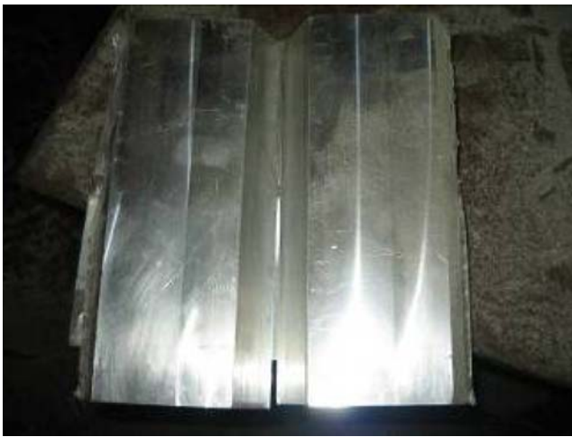
Fig. 6 Grooved for ARC welding
