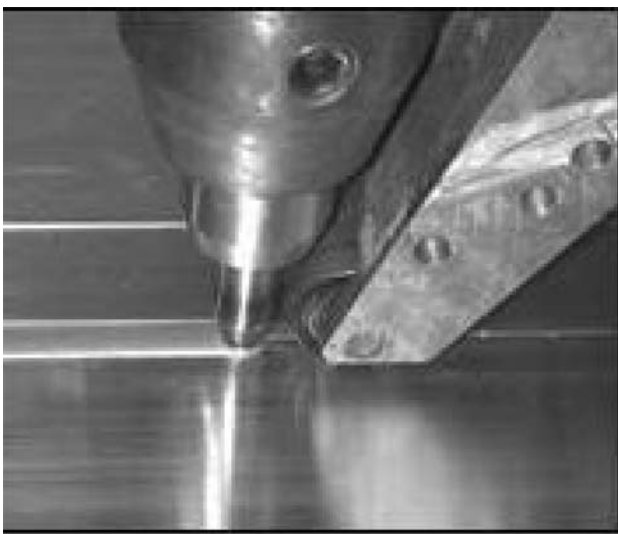
Fig. 15 Dynamic fixed roller [29]
