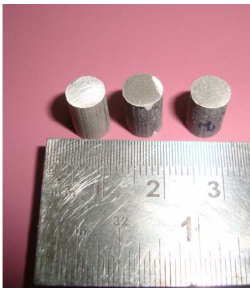
Fig. 2 Mg nano alumina composite (12 mm length and \varnothing 6.5 mm)
