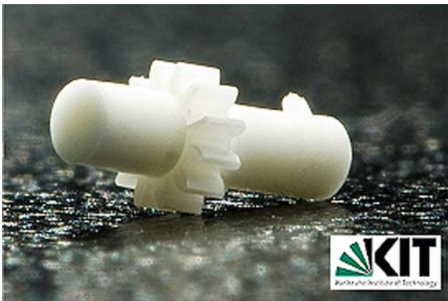
Fig. 12 Shaft-to-collar connection after sintering (fixed junction)
