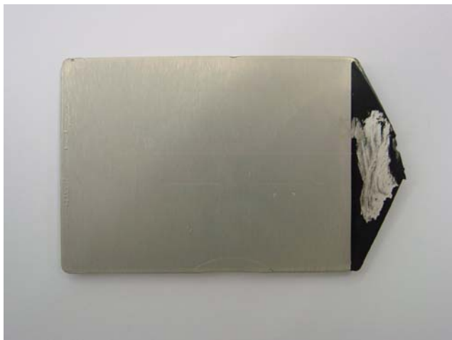
Fig. 8 Electroplating test on base plate of almost homogeneous electrical conductivity distribution (homogeneity gradient of \pm 8\Omega )
