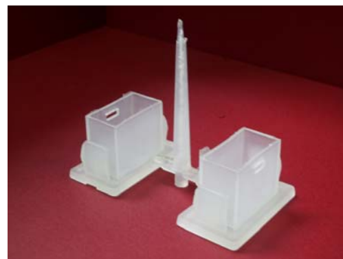
Fig. 2 The push-button housing and runner system
