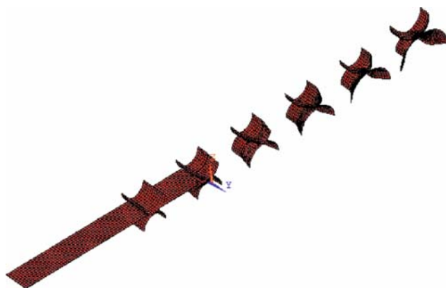
Fig. 6 V-section roll-forming model into LS-Dyna
