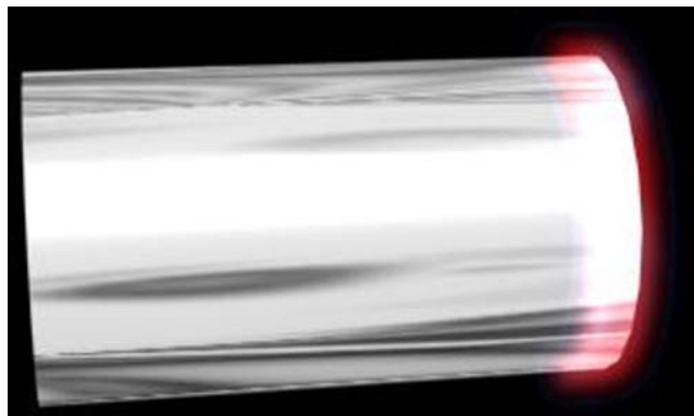
Fig. 23 Uniform heating at the tube edge (joint)
