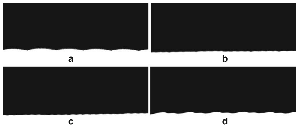
Fig. 10 Images of workpiece profile. a New tool. b After 50 min. c After 75 min. d After 175 min
