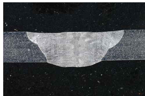
Fig. 3 Photomicrograph of a typical bead profile of a weld specimen (S20) cross-sectioned at A–A (10× magnification)
