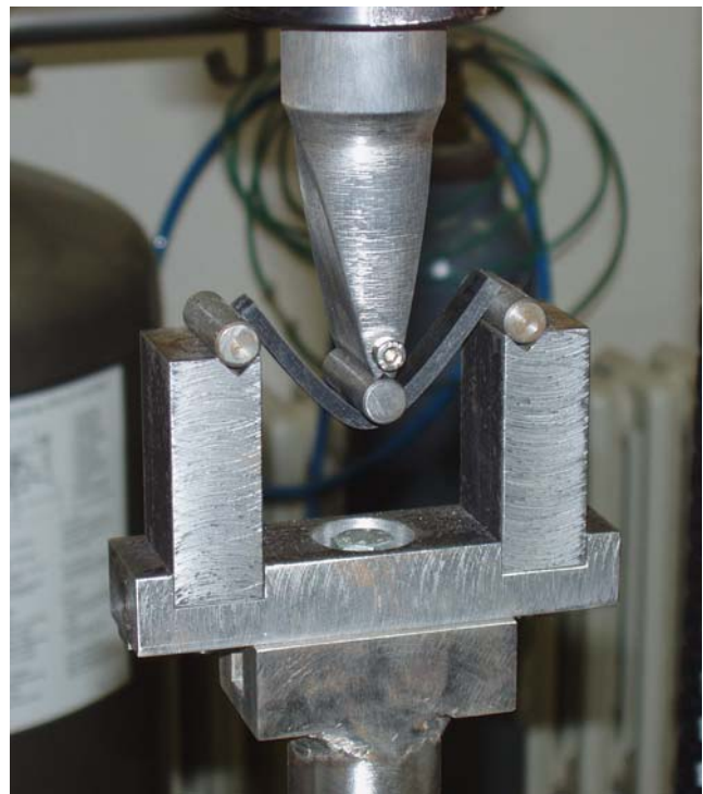
Fig. 6 Maximal bending of VeroBlack materials
