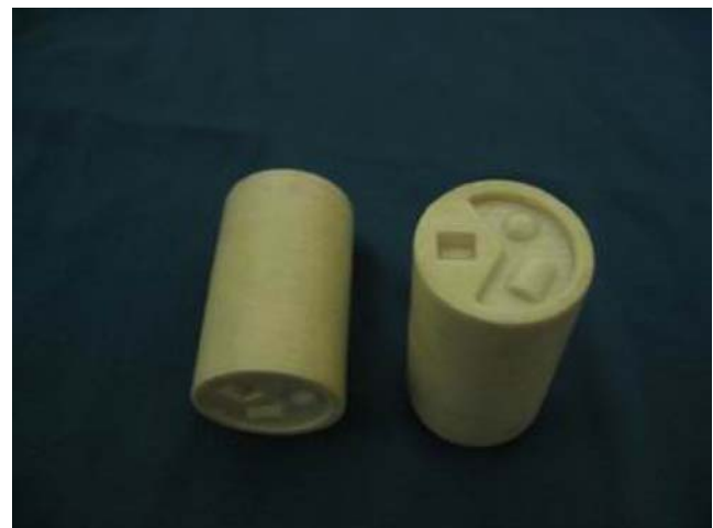
Fig. 3 Rapid prototyping gypsum powder electrode
