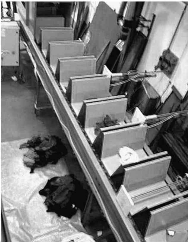
Fig. 8 Transport guide developed by the Research Centre Tecno-tessile s.r.l. in order to transport the cloths to be classified onto the measurement workbench
