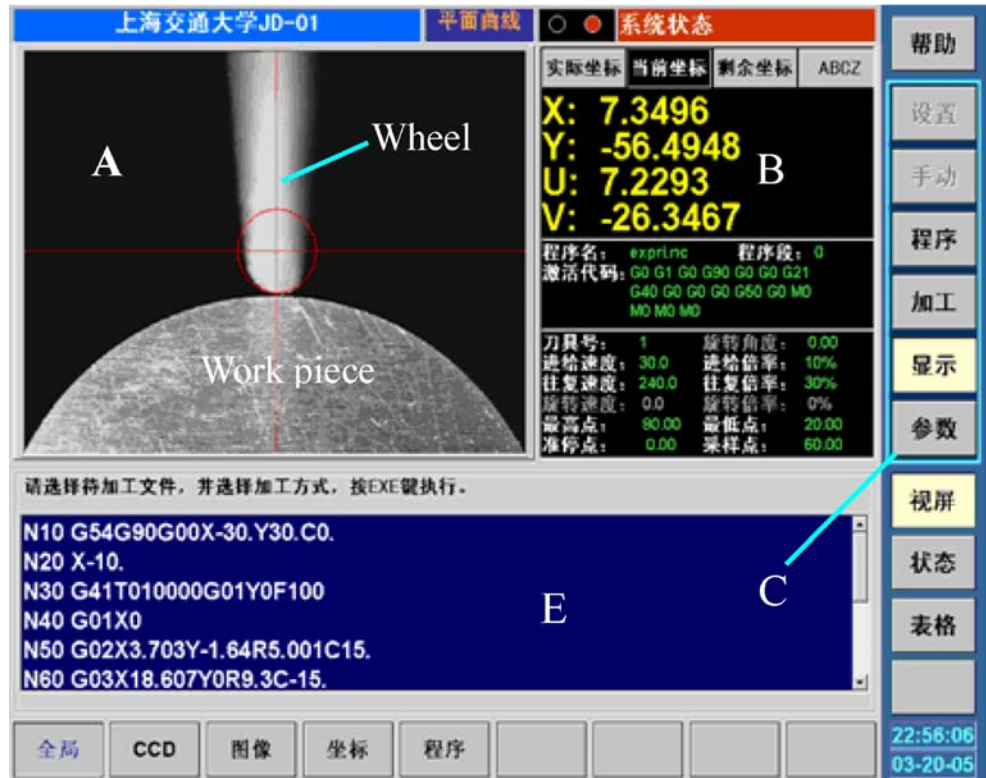
Fig. 19 The instant image during curve grinding. a Display area of work piece and grinding wheel imaging. b Display area of machine coordinates. c Operation buttons for user. e Display area of NC codes
