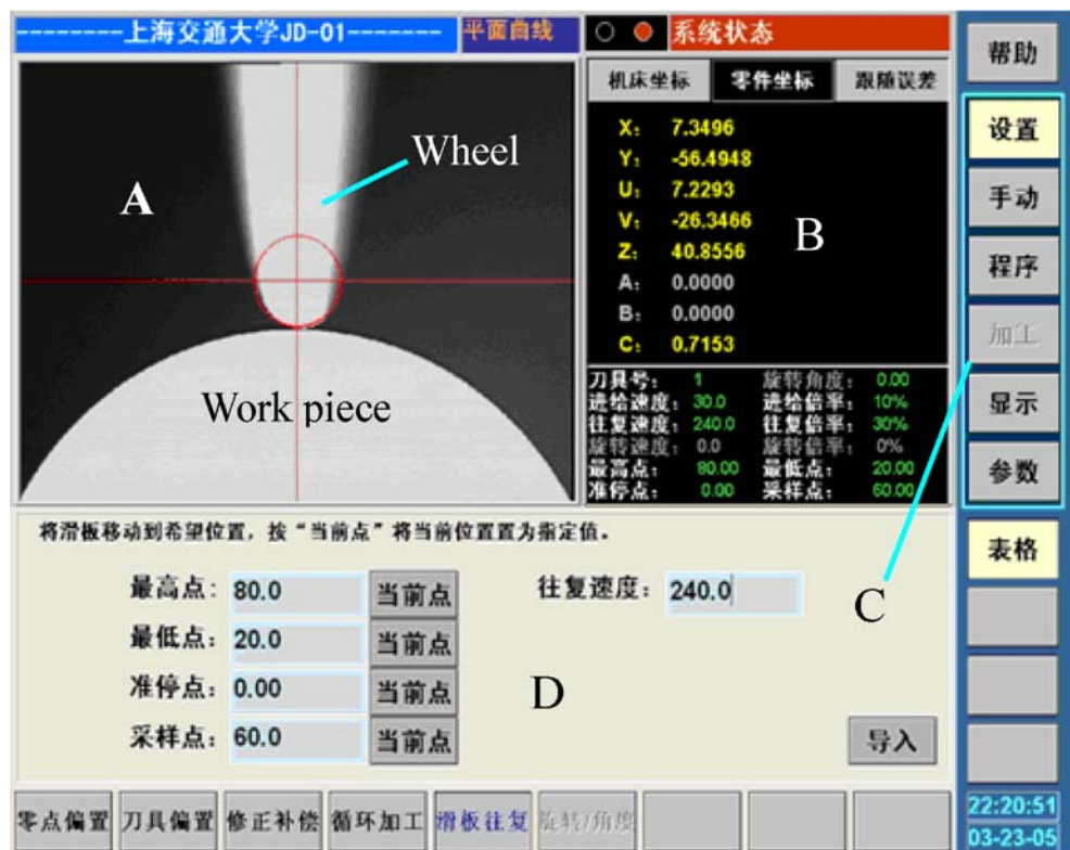
Fig. 18 Setting interface of the measurement system. a Display area of work piece and grinding wheel imaging. b Display area of machine coordinates. c Operation buttons for user. d Setting area of image sampling
