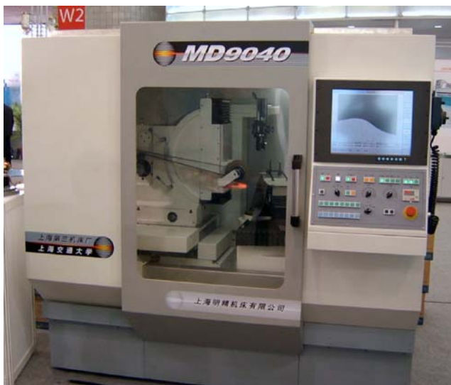
Fig. 13 MD9040 digital curve grinding machine
