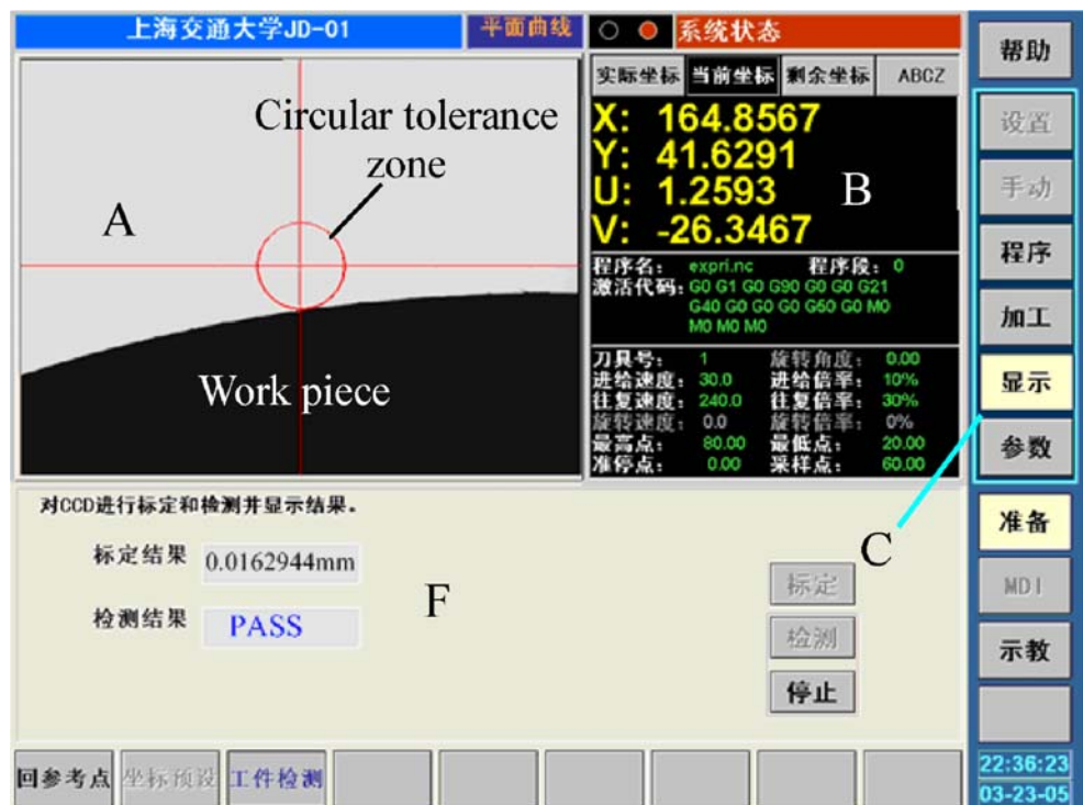
Fig. 20 The instant interface of the measurement system. a Display area of work piece and grinding wheel imaging. b Display area of machine coordinates. c Operation buttons for user. f The instant interface of detection results
