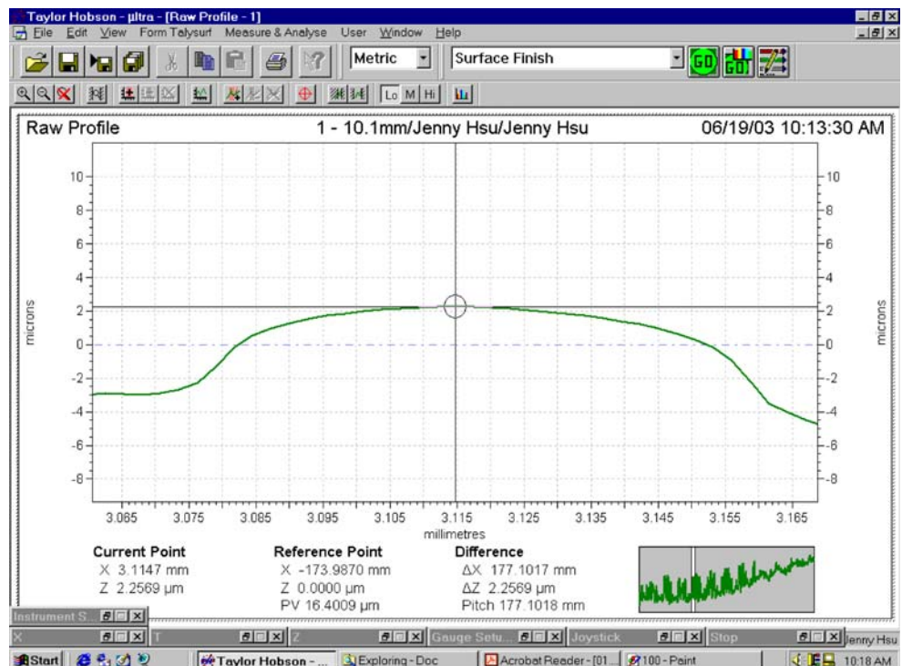
Fig. 5 Surface profile of the microlens measured using Taylor Hubson's surface profiler
