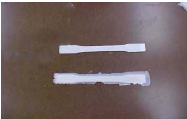
Fig. 1 Injection-molded specimen without and with flash
