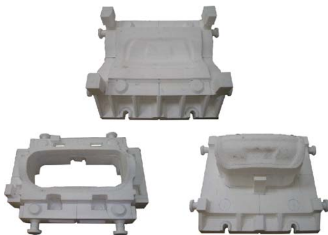
Fig. 16 The dissolve dies for drawing dies
