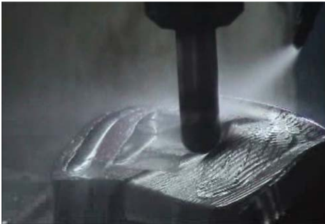
Fig. 18 CNC processing of the drawing punch
