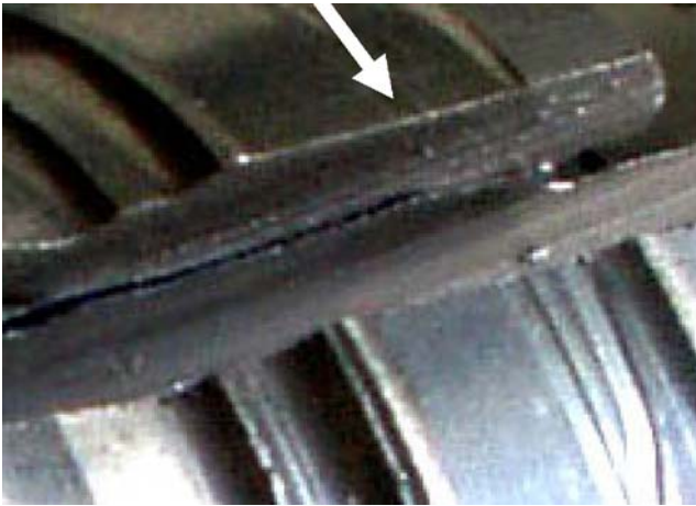
Fig. 16 Cross-section of a cross-rolled joint Type R60
