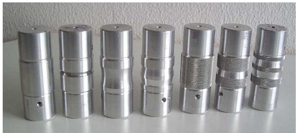
Fig. 10 Set of inserts and a variety of their contact surfaces
