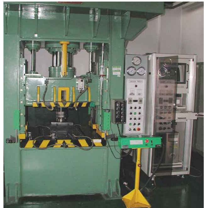
Fig. 1 Experimental equipment for elliptical deep drawing
