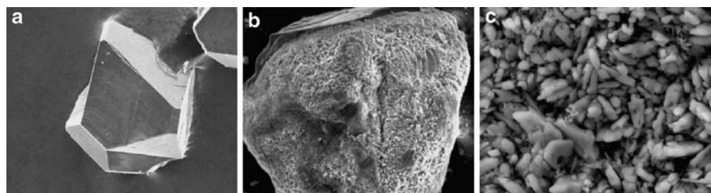
Fig. 2 SEM micrograph of CBN grain and compounds. a Original grain. b Brazed grain after etched. c Fine compounds around brazed grain
