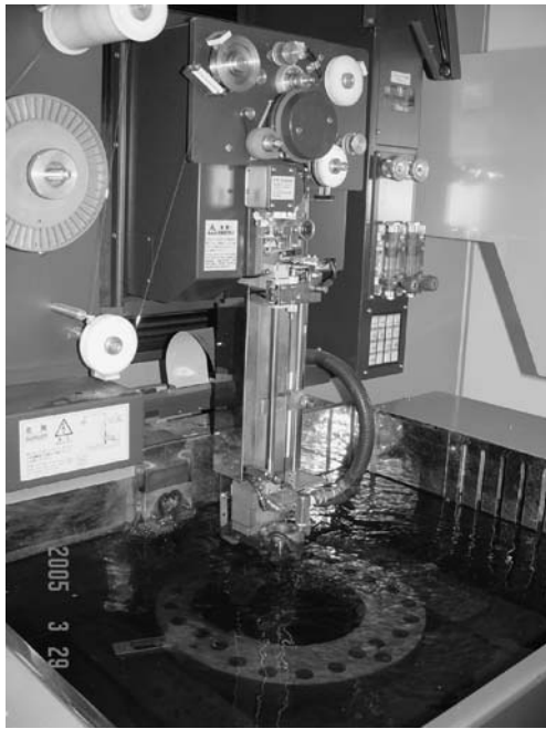
Fig. 9 Machining the square gear by electron discharge machining (EDM)
