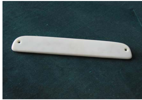
Fig. 13 FDM prototype of the car lamp veil with size 284 mm × 51 mm × 38 mm
