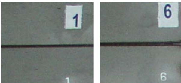
Beam Power: 580 Watts, Welding Speed: 1000 mm/min, Beam angle: 90° Beam Power: 1000 Watts, Welding Speed: 1000 mm/min, Beam angle: 90°
