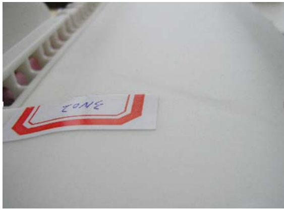
Fig. 2 The photo of sample with weldline taken by digital camera
