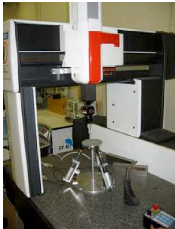
Fig. 17 Calibration of micro PKM using CMM
