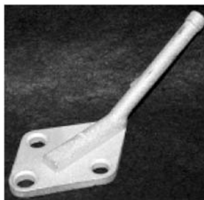
Fig. 3. The GKN Westland oil jet and eight parameters
