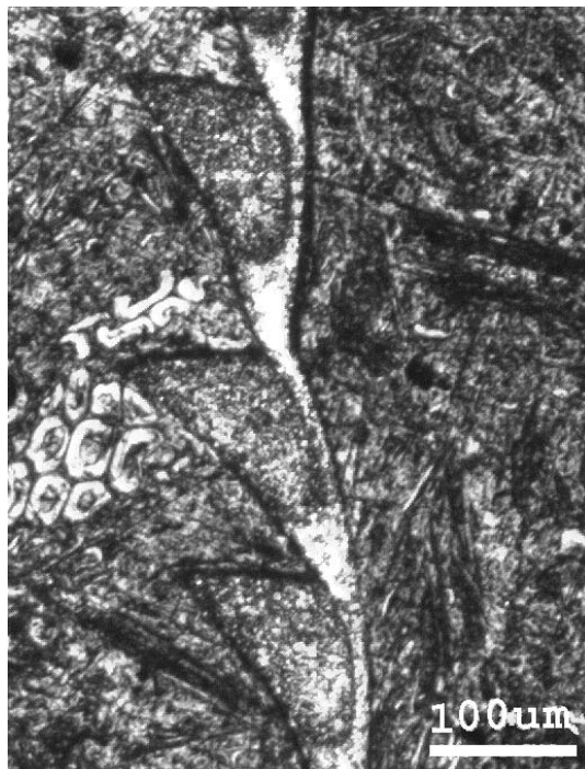
Fig. 9. Etched chip for cutting condition 2
