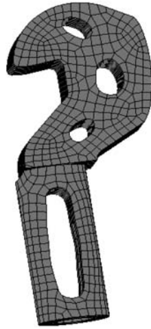
Fig. 10. Reconstructed finite element model based on the topology results
