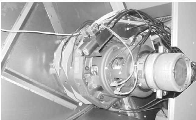
Fig. 3. Sensors on the back end of the spindle
