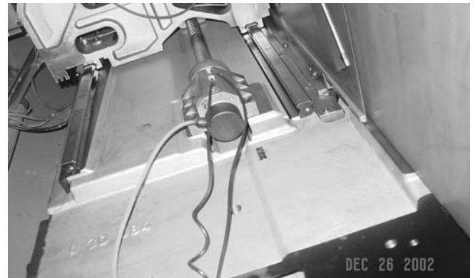
Fig. 5. Sensor on the x nut and leadscrew
