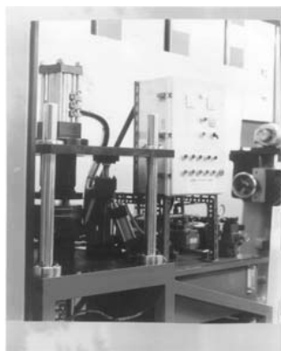
Fig. 2. Abrasive flow machine system
