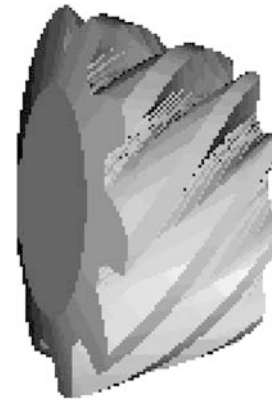
Fig. 6 The simulation result of the generated pinion
