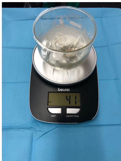
Fig. 4 Weighing scale used to weigh the cement the mixed cement before use and the discarded cement (extruded and not used)
